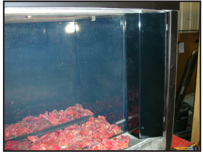
Figure 17. Outside Corner Trim Piece Installed.
